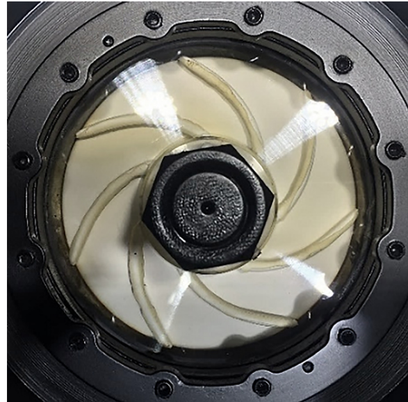
Fig. 1 Electrical submersible pump prototype with transparent shell for flow visualization
